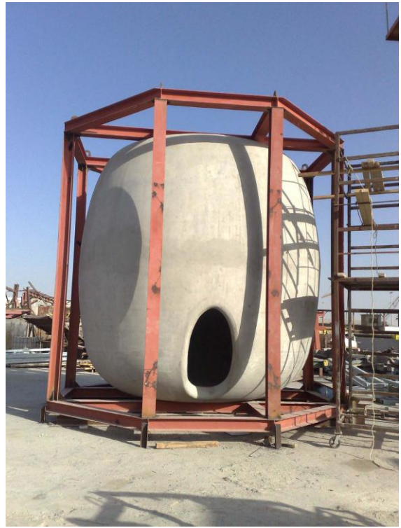
Image 15 - Glass Fibre Reinforced Concrete in a 'sandwich' construction allowed the pavilion to be constructed as a single entity
